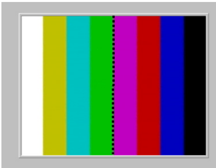
Figure 1-47. NTSC Composite Output: Standard 75 Percent Color Bars With Dot Crawl Artifact
